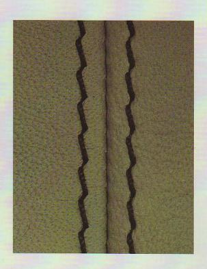
The special application needle SAN® 12 is the solution for a uniform seam appearance on both sides
